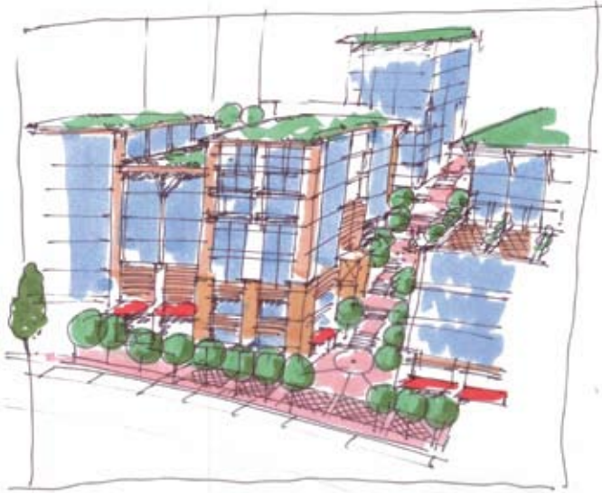
Figure 6.15 (below) Concept sketch of new, green construction along Lonsdale Avenue utilizing passive and active solar gain as well as green roofs. Drawing by Jay Hiscox.
