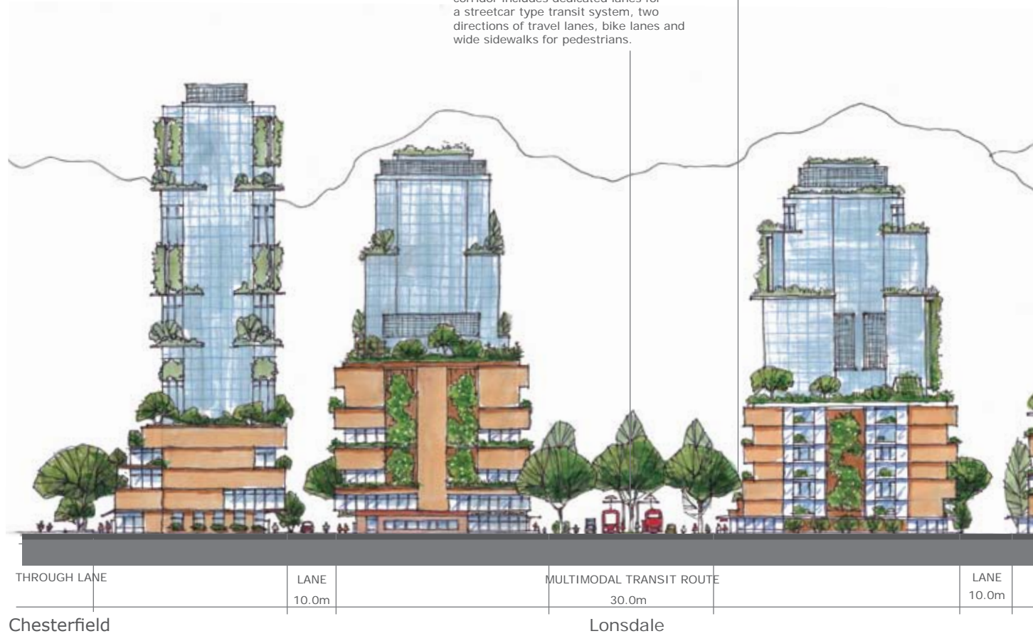
Figure 5.5 (above) Section of the Lonsdale Avenue transit corridor. Drawing by Susan Milley.
