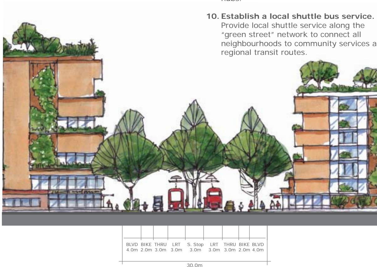
Figure 5.14 (below) Section of multimodal transit corridor with streetcar service. Drawing by Susan Milley.
