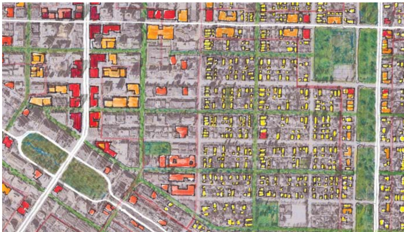
Figure 4.7 Plan detail of the charrette's "green the grid" strategy. This strategy overlays green infrastructure, including bikeways and trails, stormwater management and energy distribution over the existing public street system. "Greened" right-of-ways balance mobility needs with other service opportunities and increase connectivity between local parks, schools and other civic amenities. Drawings by Colin Cathcart, Patrick Condon, James Tuer, Daniel Roehr, Nicole Miller and Sara Muir-Owen.
