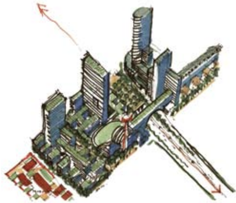
Figure 5.4 (above) The Upper Lonsdale Avenue land bridge spans the Upper Levels Highway connecting the City to the District and creating a higher density, transit-oriented development at the regional rapid transit stop. Drawing by Colin Cathcart.
