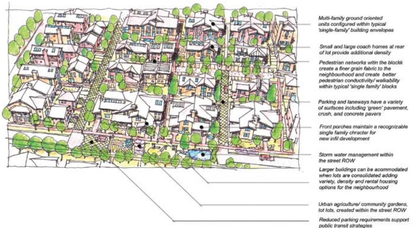
Figure 6.9 Transition single-family neighbourhoods to “ground-oriented” low-medium to medium density areas through single-family residential infill. Density is achieved by incorporating duplex, tri- and fourplex housing. Attention to building form and facade reduces the mass of larger building types and helps to maintain the high quality single-family character of the city’s core neighbourhoods. Drawing by James Tuer.
