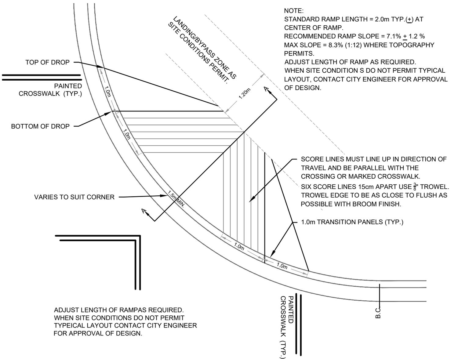
ADJUST LENGTH OF RAMP AS REQUIRED. WHEN SITE CONDITIONS DO NOT PERMIT TYPICAL LAYOUT CONTACT CITY ENGINEER FOR APPROVAL OF DESIGN.
