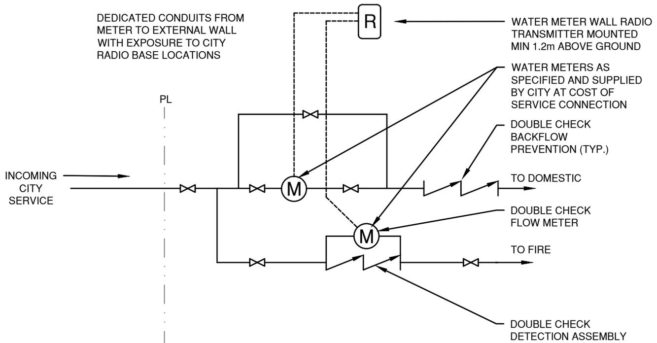
**OPTION 1: SEPARATE UNMETERED FIRE SYSTEM WITH DOUBLE CHECK DETECTOR ASSEMBLY**
