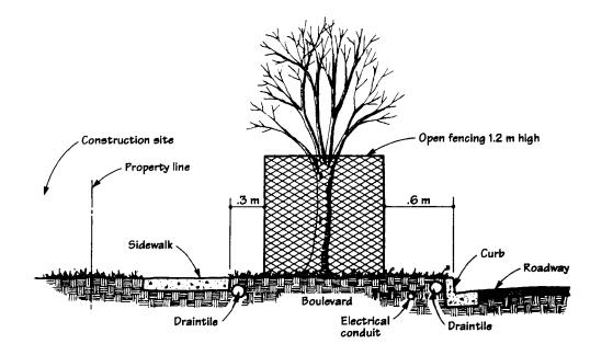
Barrier fencing used for tree protection must:
