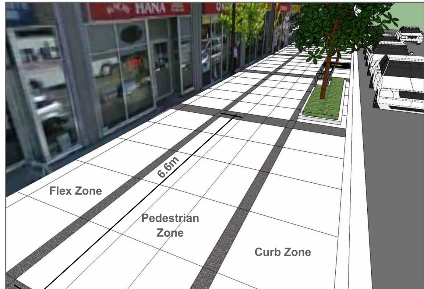
**Sidewalk Field:** Light, broom finish concrete
