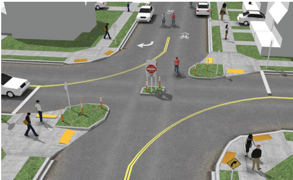
This is an example of how diagonal diverters are used. Design and implementation materials will differ at Ridgeway and crosswalks will be included.
