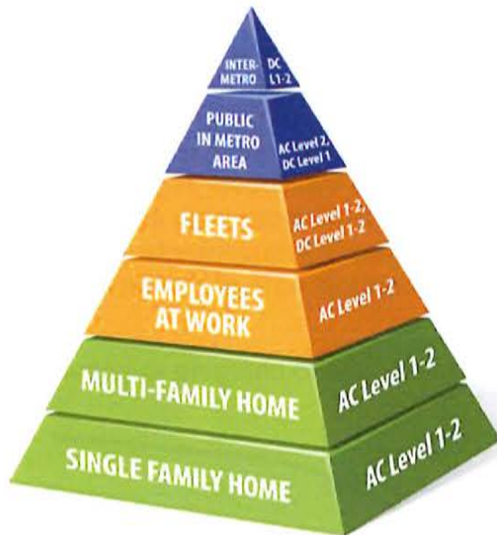
Figure 2. The EV charging pyramid, showing the role of opportunity charging in purple. (Source: Argonne National Laboratory, as presented in the City of Richmond's Residential EV Charging Local Government Guide).
