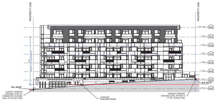
3 SOUTH ELEVATION - BUILDING HEIGHT 1/16" = 1'-0"
