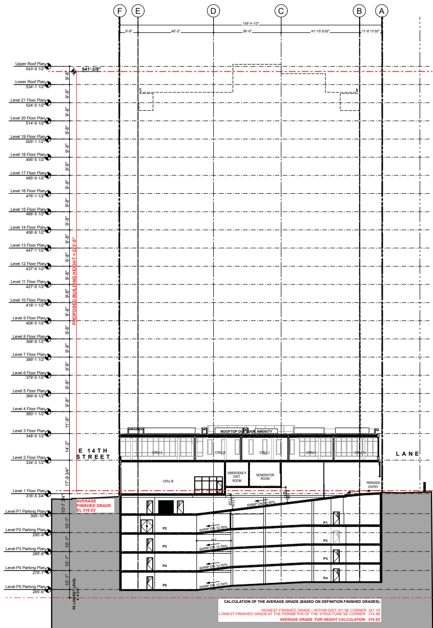
2 Building Section - North-South SCALE: 1/16" = 1'-0"
