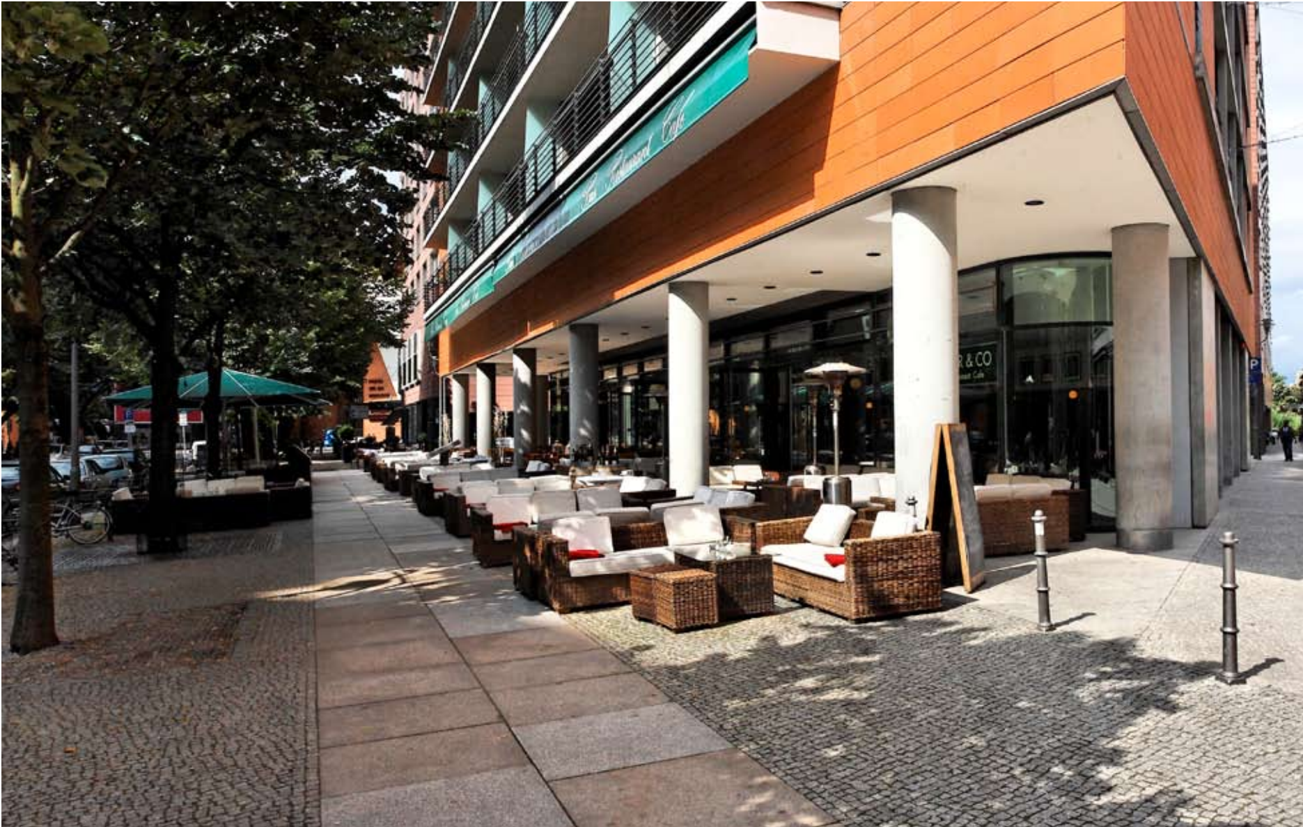
For irregular shaped sites, street level setbacks which extend from the primary Marine Drive elevation around to the secondary side elevations is strongly encouraged. This provides opportunities for additional merchandising and promotes pedestrian access onto and from secondary streets
