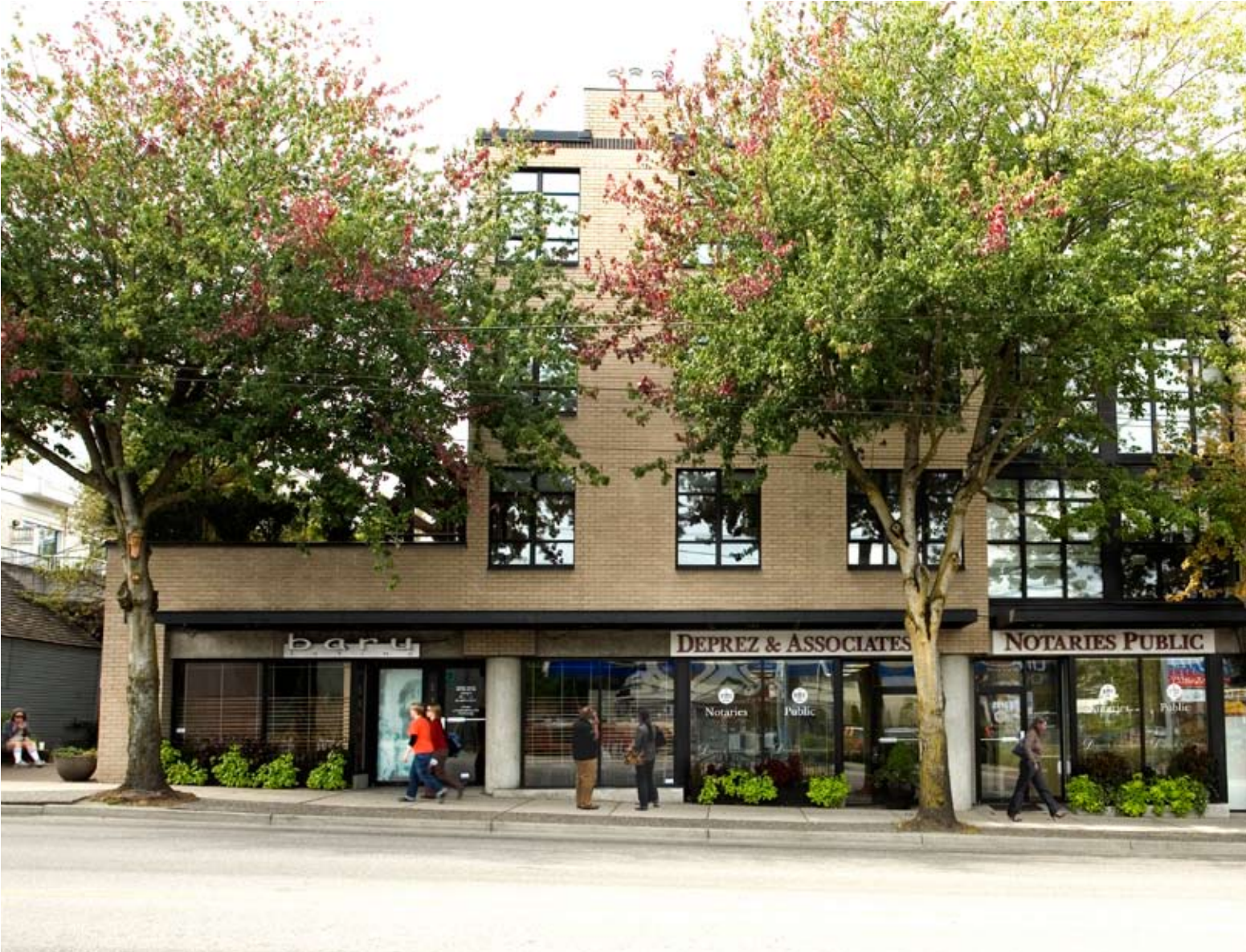
Developments to provide a cohesive framework of protection from the elements, signage, massing, detailing and materials, within which smaller retail and commercial businesses can develop their own identity. Street oriented retail and commercial units to be based on 25-35 foot module.
