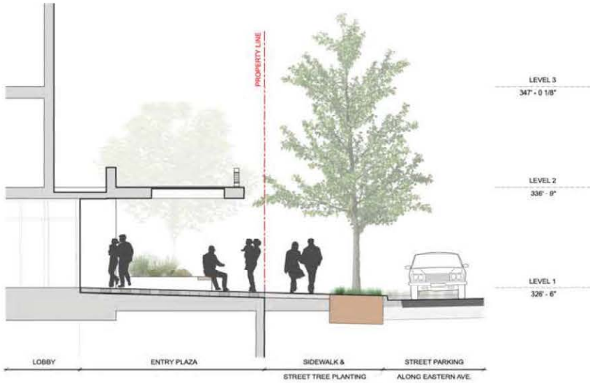
A SECTION - LEVEL 1 MAIN ENTRY Scale: 1:50
