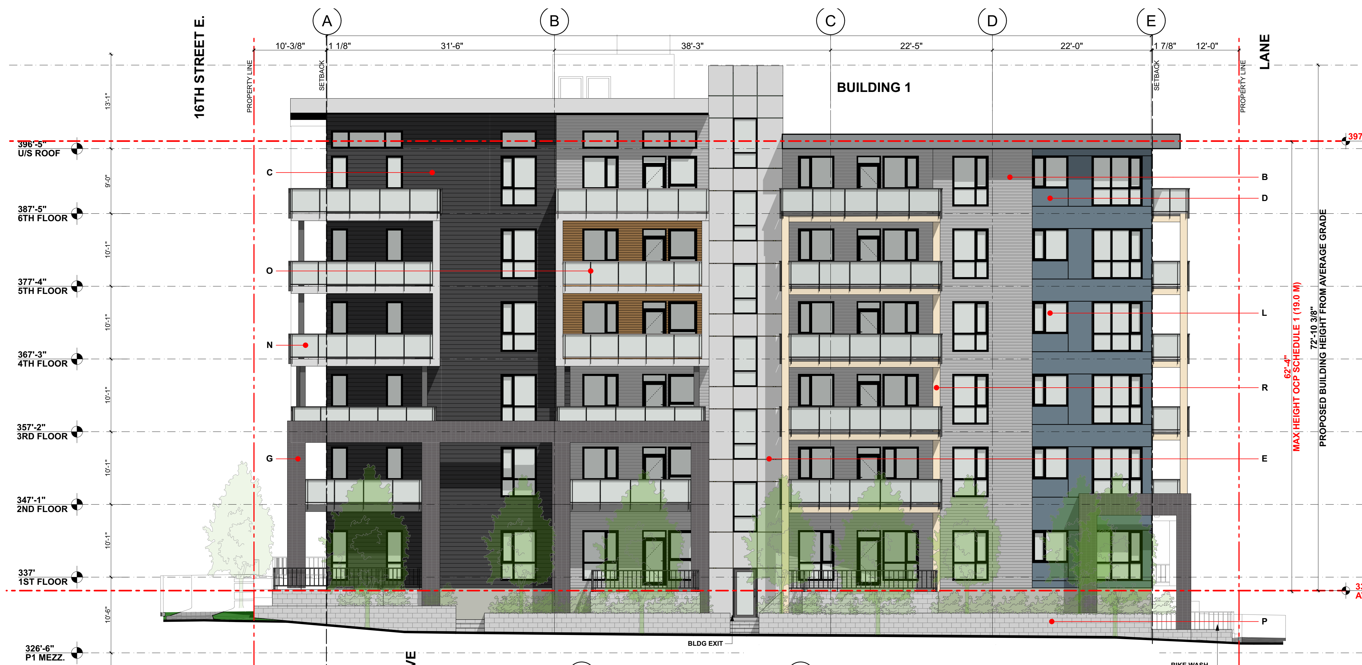
1 Building 1 - West Elevation SCALE: 1/8" = 1'-0"
