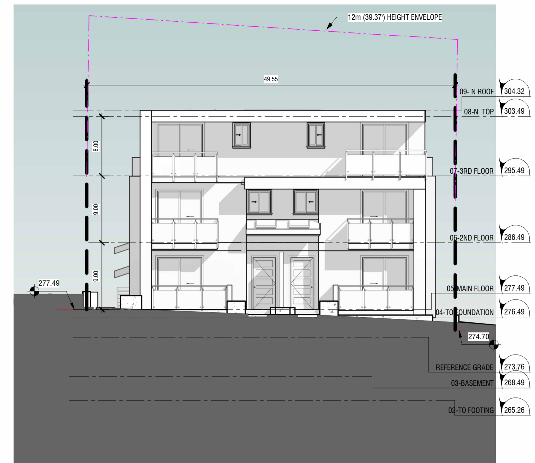
2 NORTH (FRONT) ELEVATION ELEVATION 1/8" = 1'-0"
