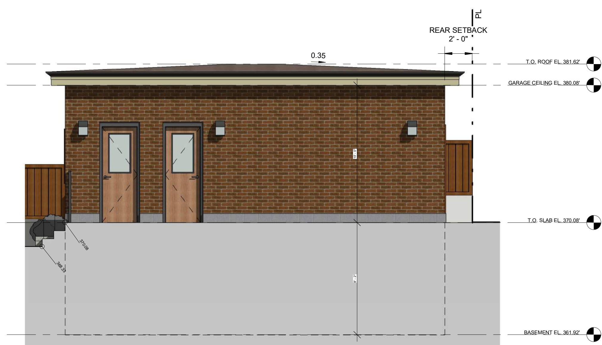
GARAGE - EAST ELEVATION - SCALE 1:50
