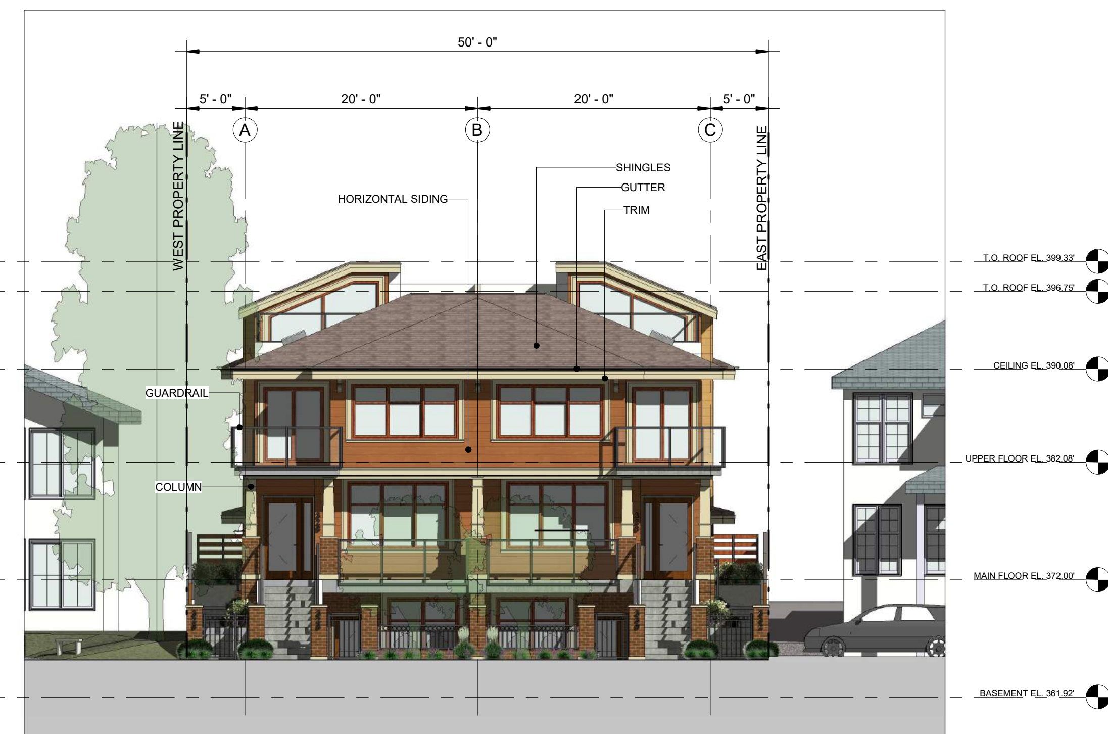
SOUTH ELEVATION - SCALE 1:100
