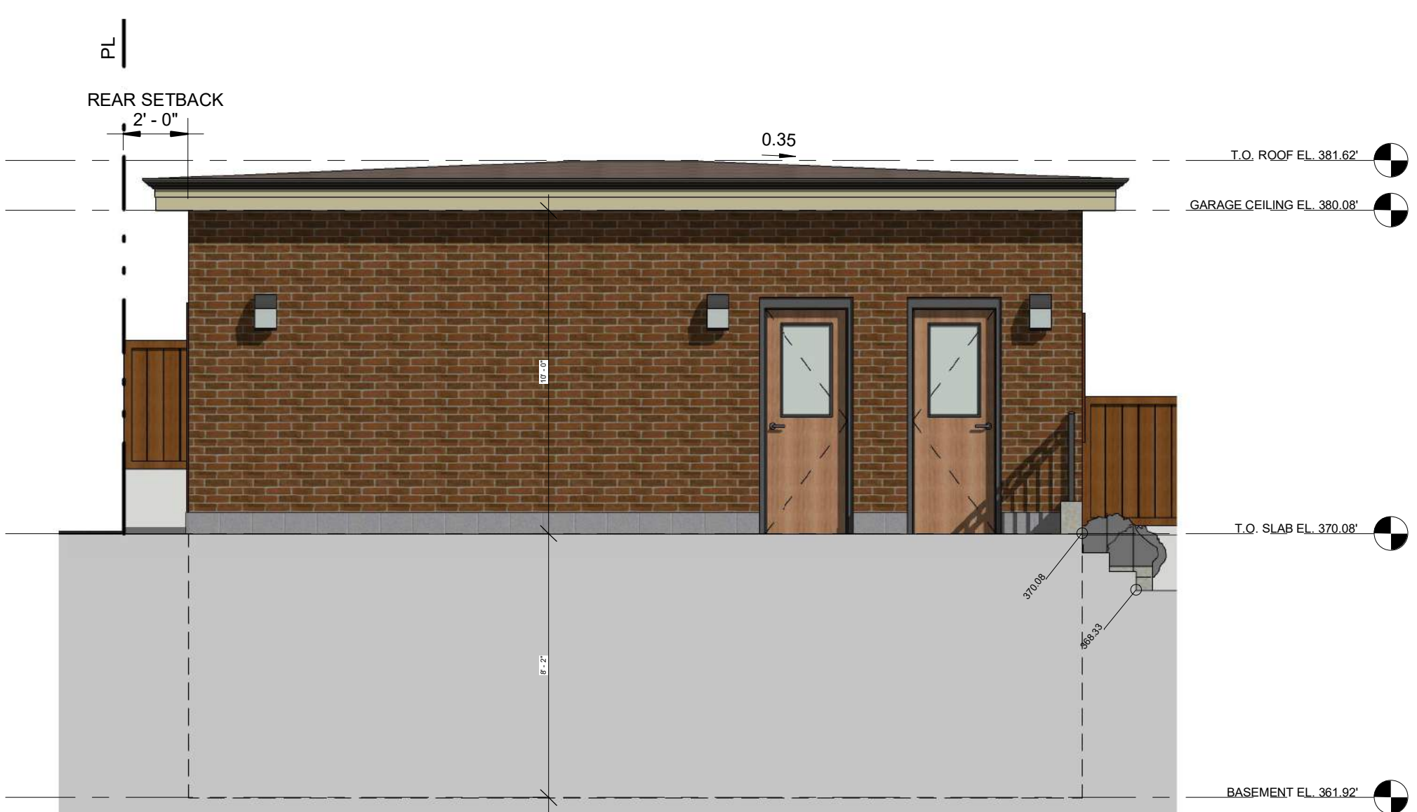
GARAGE - WEST ELEVATION - SCALE 1:50
