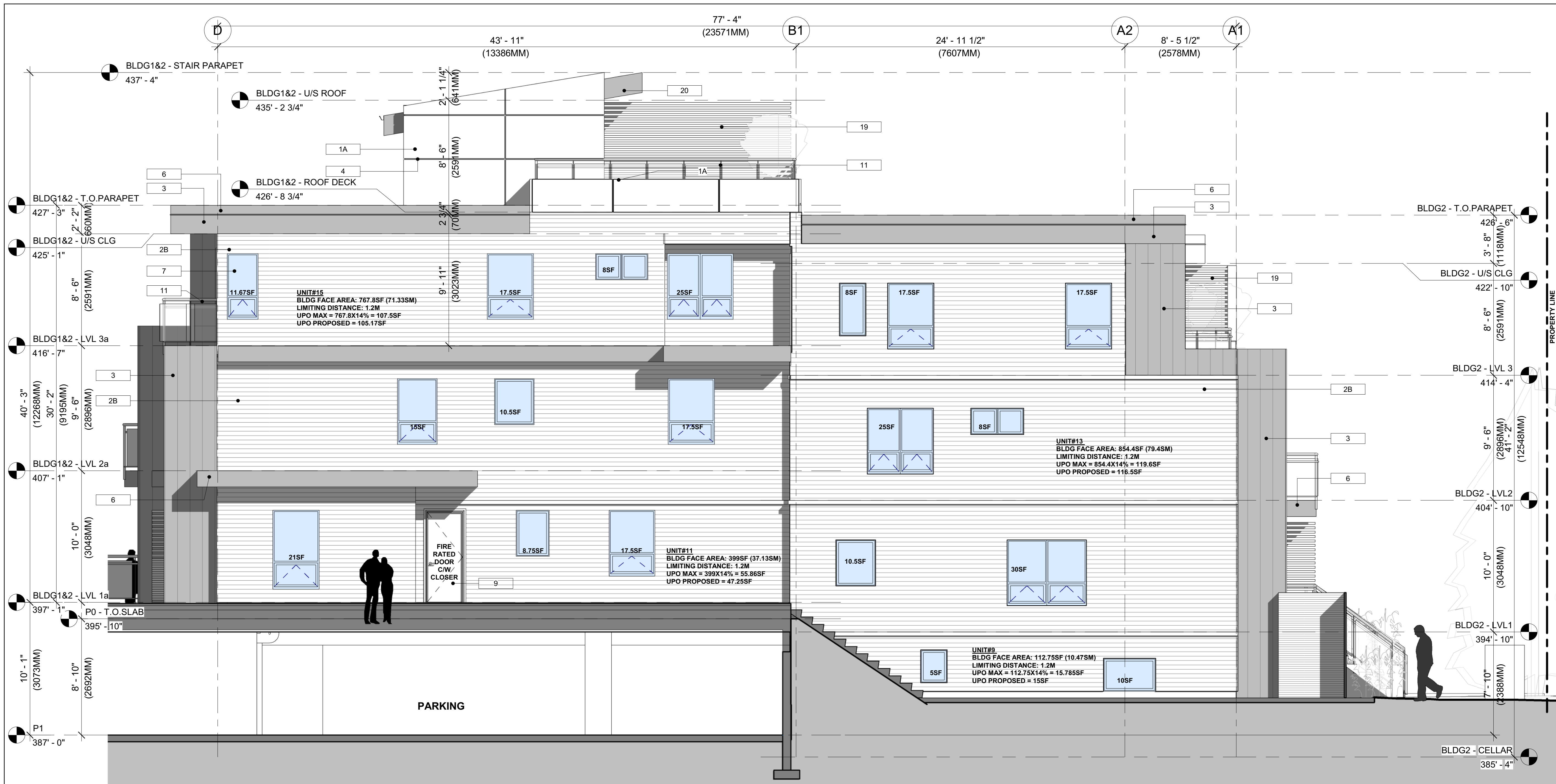
1-4 NORTH ELEVATION BLDG#2 1/4" = 1'-0"
